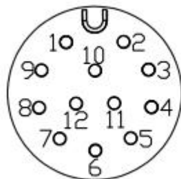
Fig. 34 Definition of LAN port pins
